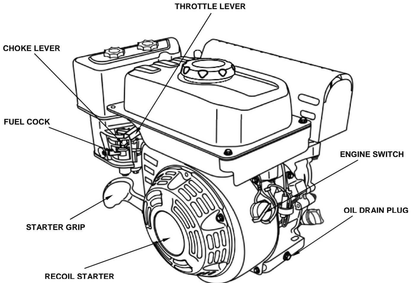
**Fuel cock:** a switch in the fuel line to control the fuel flow in the fuel line.
