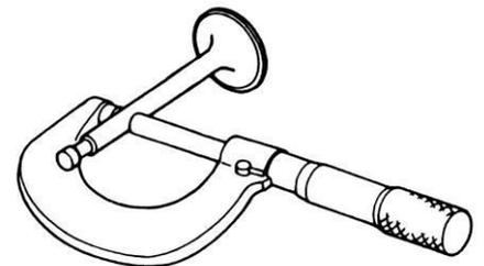
Replace the valves if their OD is smaller than the service limit.
