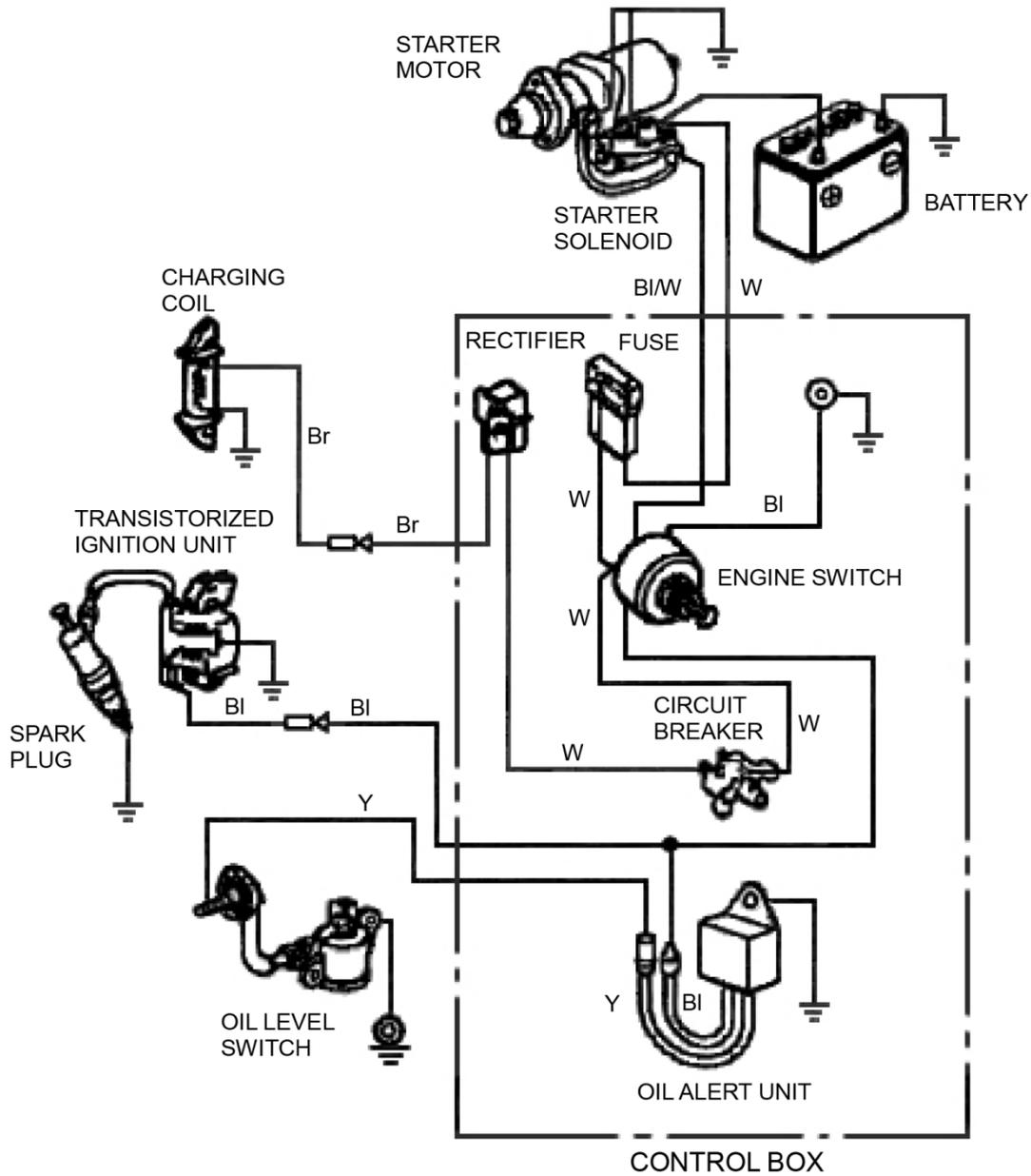
Engine Type with Oil Alert and Without Electric Starting
