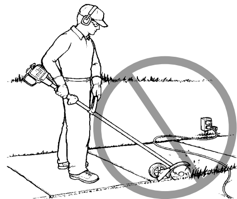
Prohibition - Edger Operation w/Electric Cord on Ground
